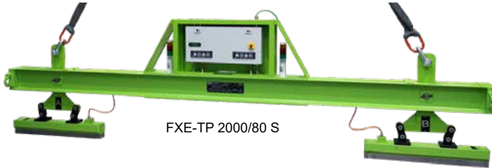
FXE-T Electro-Permanent Deep field Truss
