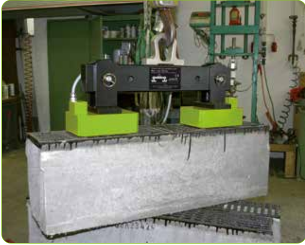
FXE-T Electro-Permanent Deep field Truss
